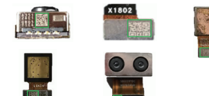
Micro QR codes laser-engraved on metallic surfaces
