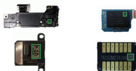
Micro QR codes laser-engraved on PCB surfaces
